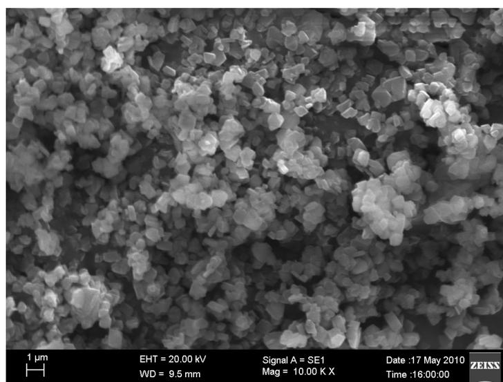
**Fig.3:** SEM image of silver nanoparticles formed by *Euphorbia hirta* L
