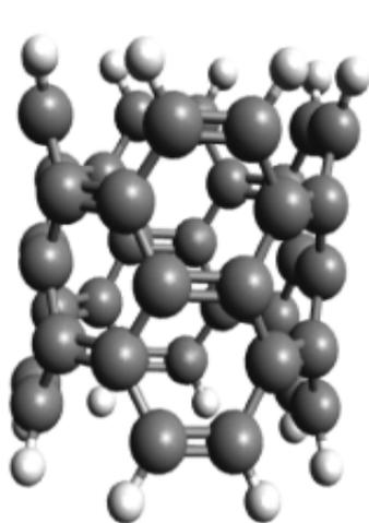
Figure 1. The structure of carbon nanotube, zigzag.
