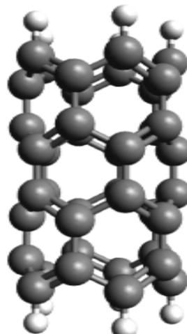
Figure 2. The structure of carbon nanotube, armchair.
