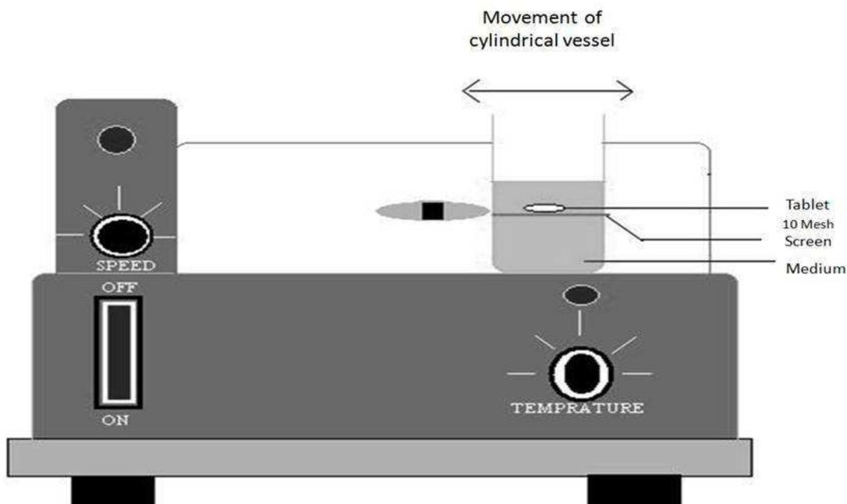
Figure 1: Device used to determine the disintegration time of fast dissolving tablets
