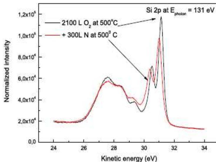
**Fig. 2 Nitridation of the silicon sample at different oxide thickness on the silicon substrate**
