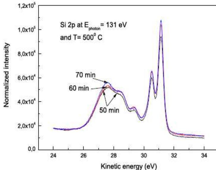
**Fig.1 Oxidation of the silicon sample at 60 and 70 minutes**
