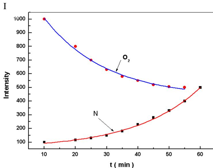
**Fig. 3 The oxynitride growth behavior with atomic nitrogen and molecular oxygen**
