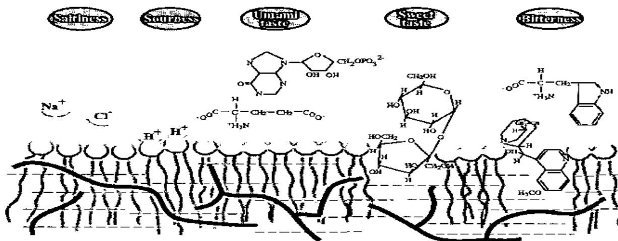
**Fig. 4:** Interaction between chemical substances to produce taste and lipid/polymer membrane. MSG and IMP are shown in umami taste, quinine and L tryptophan being shown in bitter taste.
