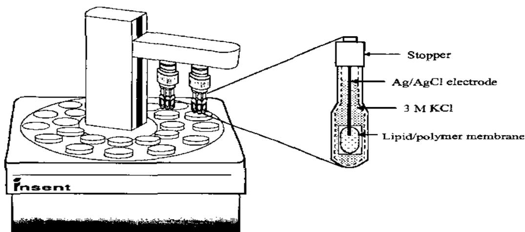
**Fig. 3: Commercially sold taste-sensing system (SA402BJ Intelligent Sensor Technology, Inc.).**
