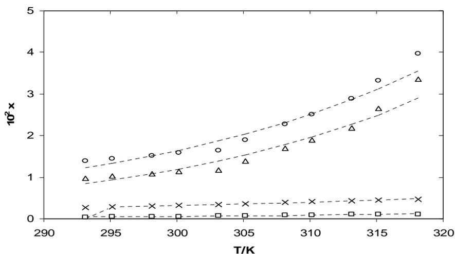
**Figure 3: Solubility  $x$  of cholesterol as a function of temperature in methanol;  $\square$ , ethanol;  $\times$ , propanol;  $\Delta$  and butanol;  $\circ$ .**
