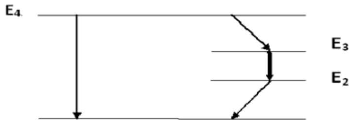
Fig III: four level laser
