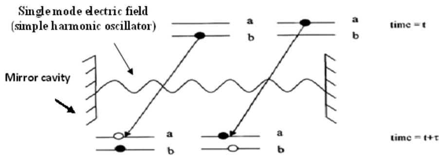
Fig I: A Cavity with two mirrors
